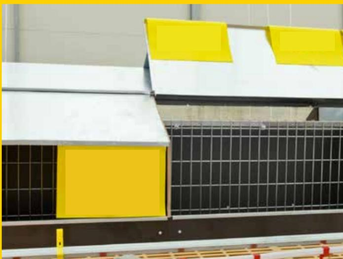
The eggs collection occurs through the egg belt of 500mm, or 250mm in case of wall nests, that runs in the middle of the automatic nests. The belt is made of pure polypropylene and furnished with holes designed to avoid the movement of the eggs on the belt while it is working.
