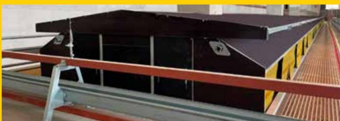
Our FAMILY NEST has an automatic expulsion system, activated by an engine installed between the rows of nests, that is set from the central control panel in order to work at a specific time of the day. The expulsion system has a wire mesh, divided in two parts, that gently pushes the birds out of the nest. Once the nest is closed, the birds cannot get in until it's opened again. This allows to regulate the entrance to the nests according to the desired time.
