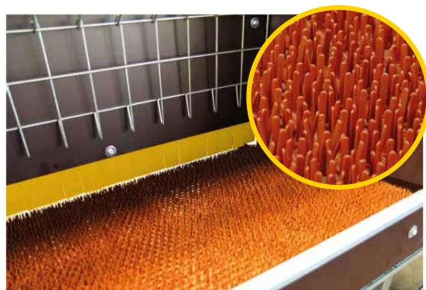
To guarantee the best possible comfort to the birds we equipped our nests with an Astroturf mat, that has the double advantage to provide the feeling of natural grass and, at the same time, facilitate the internal cleanness of the nest. The mat doesn't hold the dirty, which can easily pass through it once dried, and can be simply removed to facilitate the cleaning procedures.
